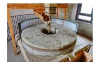
The "rotating" wheel on top is made of Sidobre granite, while the "dormant" wheel in the wood formwork is made of flint.
